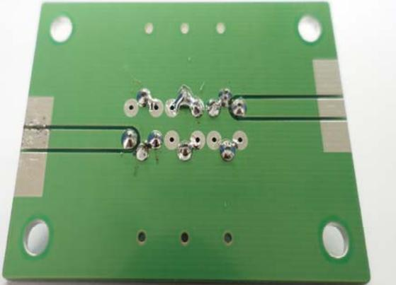
The back of the green PCB showing the soldering process. Solder wire is being applied to the shell feet and pins of the filter component.                      | <p>2. Turn PCB to the back (solder side). Melting solder wire with soldering iron. Then solder shell feet and pin in circuit diagram of PCB. (Note: The soldering temperature should not be too high. Soldering time should not take too long. Soldering contact about 1-2 seconds.)</p> |
