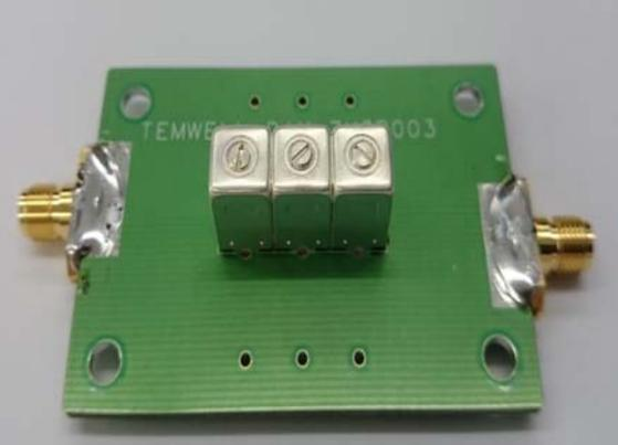
The front view of the PCB after SMA connectors have been soldered to the shell feet. The connectors are gold-colored and mounted on the left and right sides. | <p>3. Soldering SMA connector at the place marked on PCB. (Note: In order to prevent cold solder when grounding soldering, adhere tin as much as possible on the solder side between connector and PCB.)</p>                                                                             |
