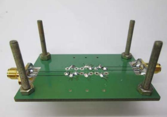
The back view of the PCB showing four long screws and hexagon nuts used to secure the board. The screws are inserted into the four corner holes of the PCB.   | <p>4. Long screws and hexagon nuts lock into four corners of PCB.</p>                                                                                                                                                                                                                    |
