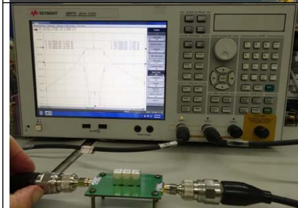
6. Connect DIY Test Circuit to Network Analyzer to make measurements.
