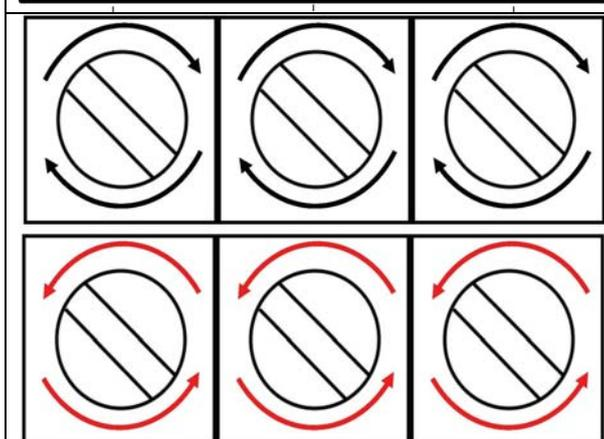
8. Tuning all screws with same direction, distance, angle and the numbers of times. The curve will shift from the original Center Frequency to the one you want. The filter can be adjusted +/- 5MHz.
