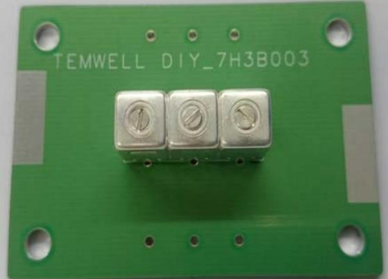
A green PCB with the text "TEMWELL DIY_7H3B003" printed on it. A silver helical filter component is mounted in the center, with three shell feet visible.       | <p>1. Insert Helical Filter into PCB component side (PCB logo face up). Please pay attention to whether shell feet and pin was tight inserted into PCB hole.</p>                                                                                                                         |
