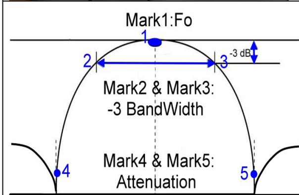
7. Set up Network Analyzer to measure parameters of Center Frequency ( $F_o$ ), Bandwidth (BW), Rejection (Attenuation), Insertion loss (IL) and Return Loss (RL).
